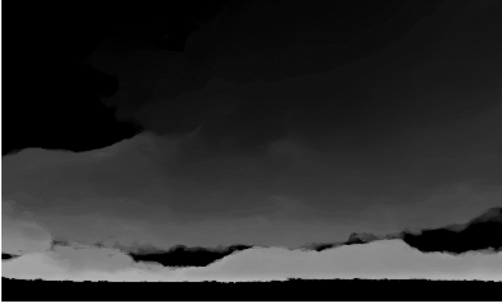
Figure 42: Weighted mean of cloud samples depth. This depth is used to sample the aerial perspective scattering and transmittance applied on clouds as a post-process.
