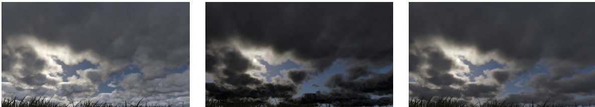
Figure 35: Issues when integrating scattered light with left: ( S ) is executed before ( T ) (not energy conservative), middle: ( T ) is executed before ( S ) (too much absorption of energy), right: a reference integration with many step showing the expect result.
