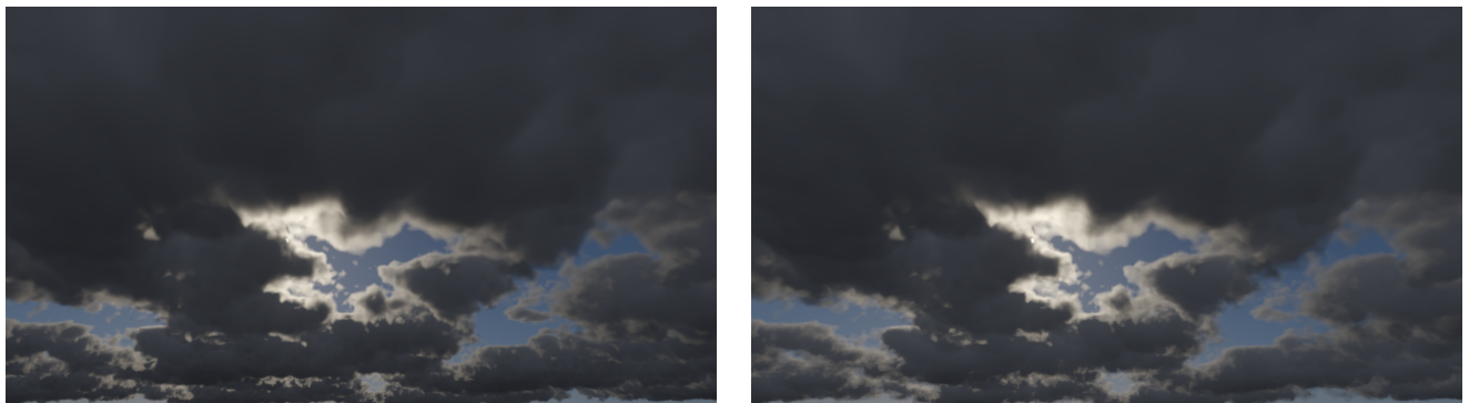
Figure 37: Left: Rendering clouds without Equation 17: 512 samples are needed to converge, and Right: with Equation 17 improved integration showing only 21 samples are needed to converge to an correct/acceptable visual result.
