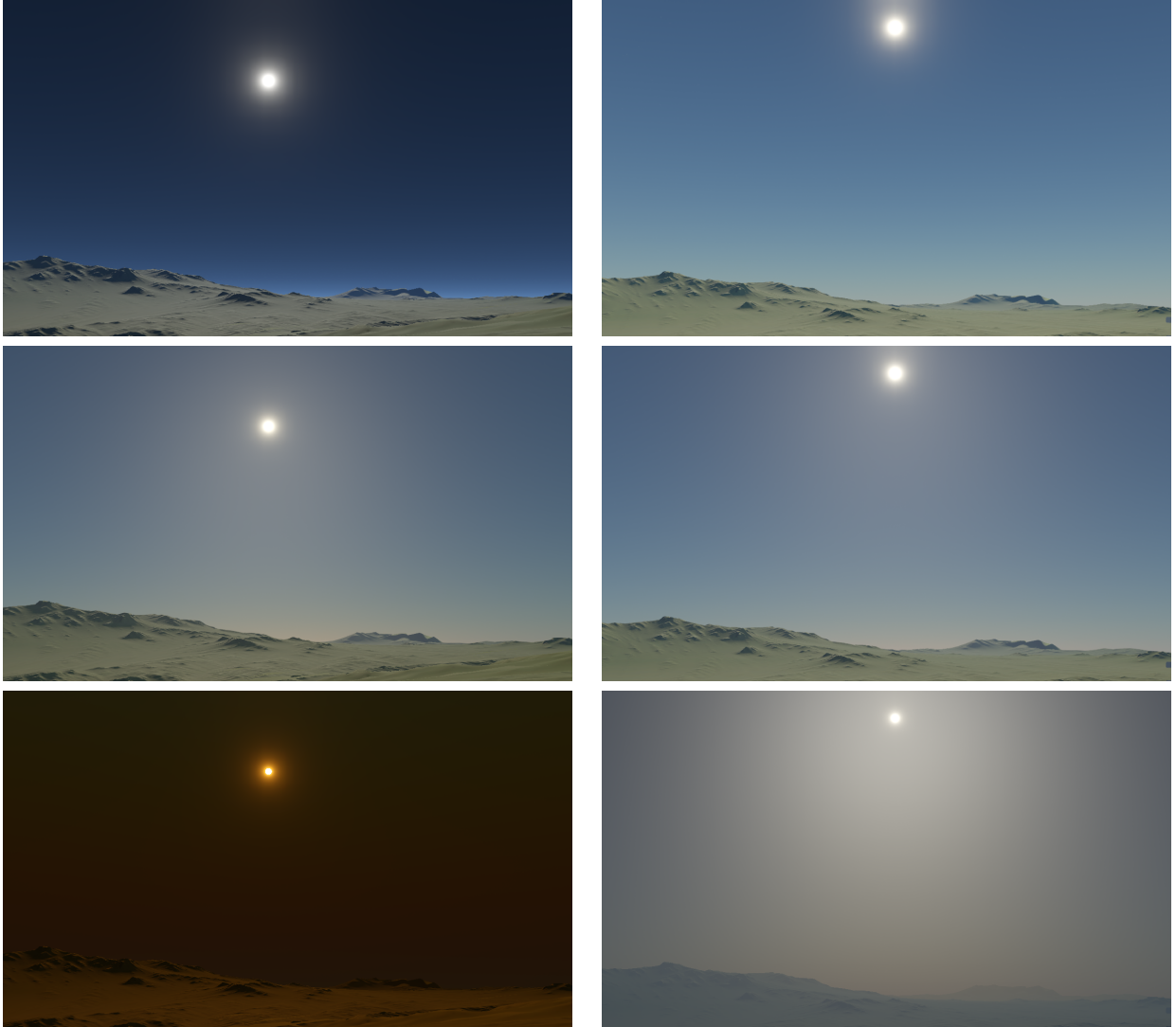
Figure 15: Left: light, earth-like and heavy Rayleigh scattering. Right: default earth-like sky with no, default and heavy Mie scattering.
