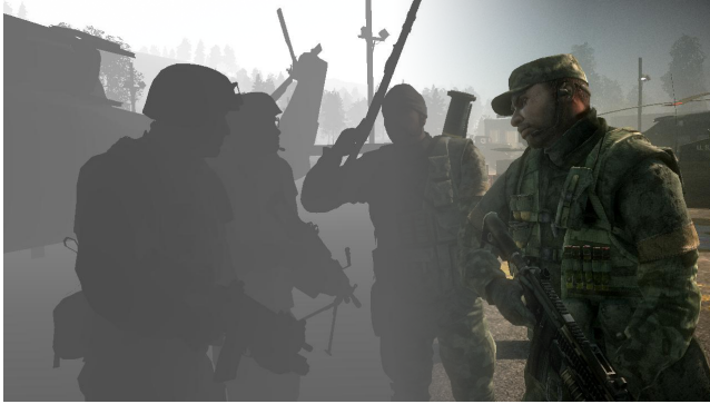
Figure 2.1. Depth and color. Linear grayscale depth map on left (white is far away), color image for the same scene on the right.
